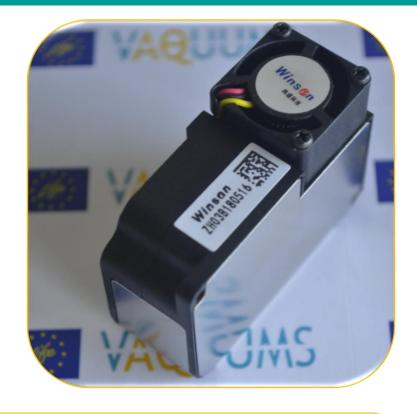
The Winsen ZH03B is a small size sensor. It uses a laser to detect dust particles in the air according to the light scattering principle. It can measure PM1, PM 2.5 and PM10. It is used in air quality monitoring equipment, air purifiers, ventilation systems, air conditioner, and smart home equipment.
